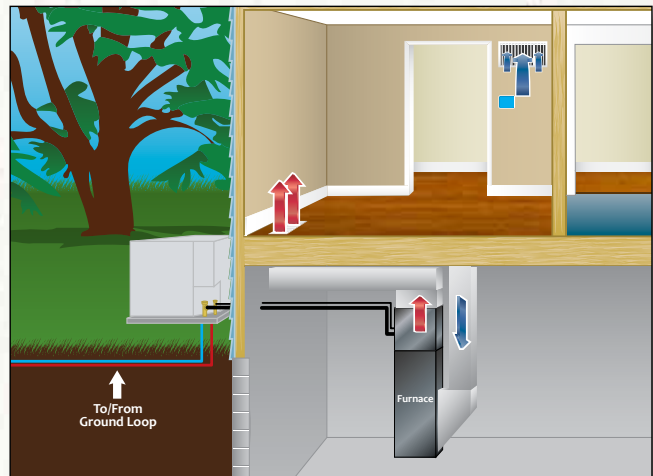
Common hybrid heating system with furnace.
