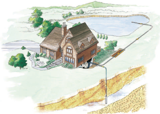
Open Loop: Well water from an existing well can be used, then discharged into a drainage ditch or pond.
